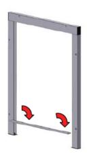
2.2.9. Fix on the floor the "bottom track" using references on both bottom corners (accessories).
